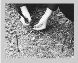
Even after you've strung out your trench, it's possible for the string to move (or, more likely, for some unfortunate person to trip over it or kick the pegs out of alignment). To make it easier to reconstruct the precise location of your original corners, mark the place where the strings cross with a permanent, easily visible pen line. In this way, if the string is ever moved, you'll be able to see its original position easily and replace it accordingly.
